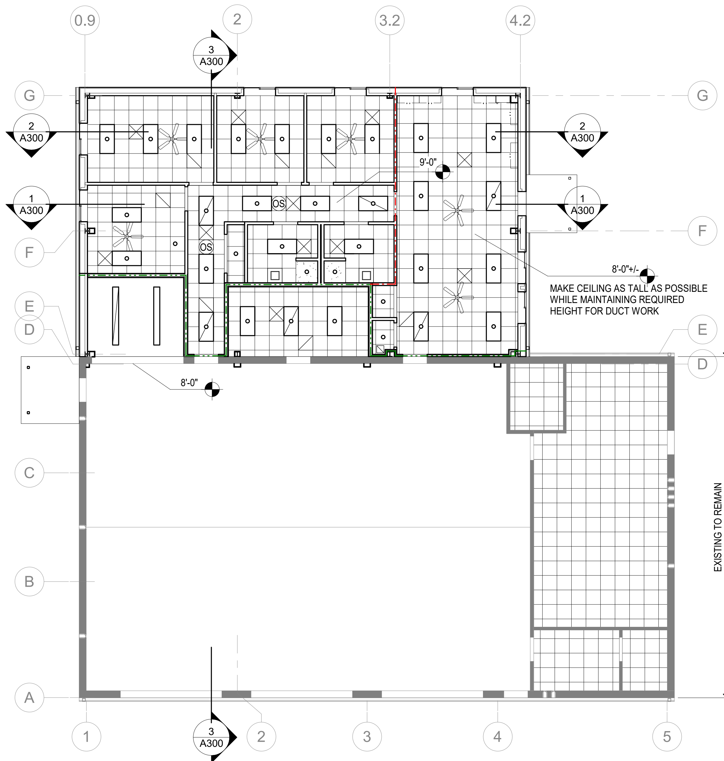
2 FIRST FLOOR REFLECTED CEILING PLAN A101 SCALE: 1/8" = 1'-0"
